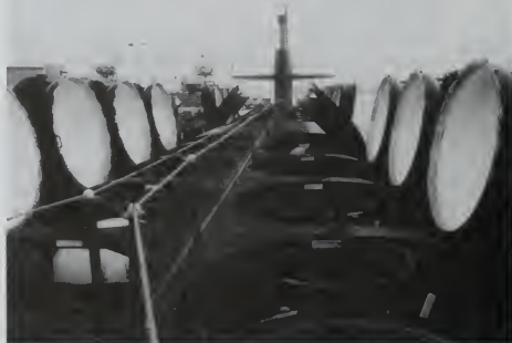
Figure 35: USS Ohio , strategic nuclear submarine of the U.S. Navy. Commissioned in 1981, it carries 24 Trident ballistic missiles in a double row of vertical launch tubes (shown with hatches open). The average patrol time at sea of Ohio-class submarines is 70 days, and their nuclear reactor cores need replacement only once every nine years.
